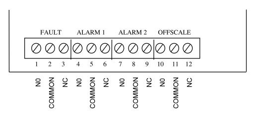
Figure 3 - Controller Lower Circuit Board
