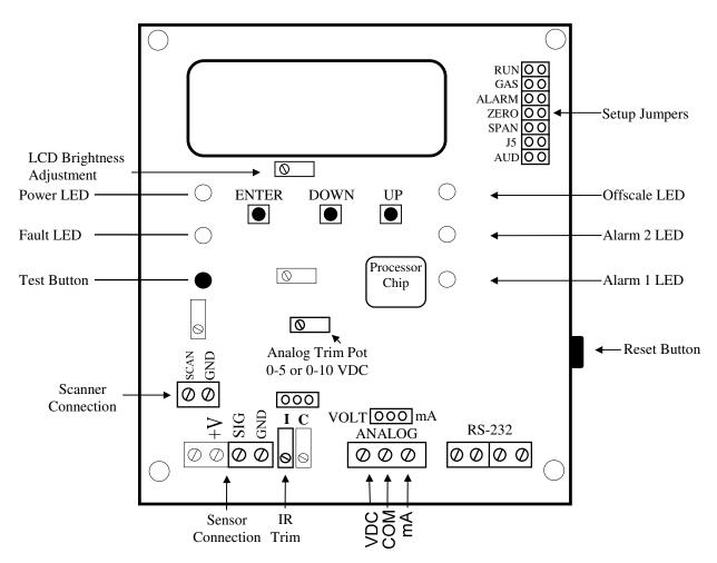
Figure 2 - Controller Upper Circuit Board
