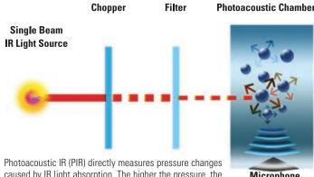
caused by IR light absorption. The higher the pressure, the greater the concentration of measured gas.
