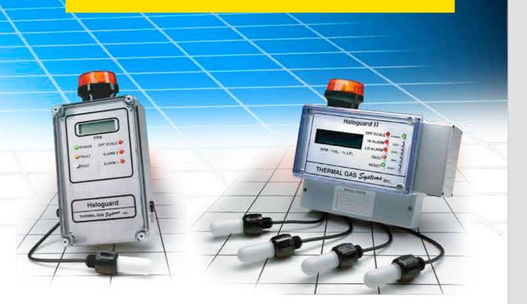
Haloguard CMOS Fixed Gas Monitors feature two adjustable alarm levels between 10% and 100% of scale, and two additional alarms for fault and offscale conditions. Options include: battery backup, strobe and audible alarms. Solid state electronics ensure dependability. Sensors can be located up to 300 feet from the controller.
